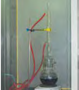
Korozyon Testi / Corrosion Test TS 3156 EN ISO 3651-1 / (ASTM A262 Practice C) TS 3157 EN ISO 3651-2 / (ASTM A262 Practice E)
