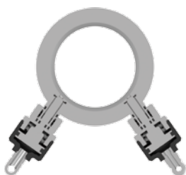
Arrangement of the flushing valves
