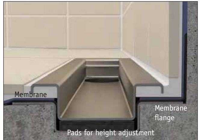
Tiles and liquid membrane
