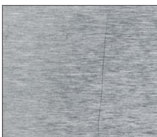
Surface finish: fine-machined and grinded, R_a 0.4 \mu m
