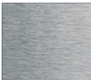
Surface finish: fine-machined, R_a 0.8 \mu m
