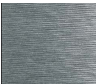
Surface finish: machined, R_a 1.2 \mu m
