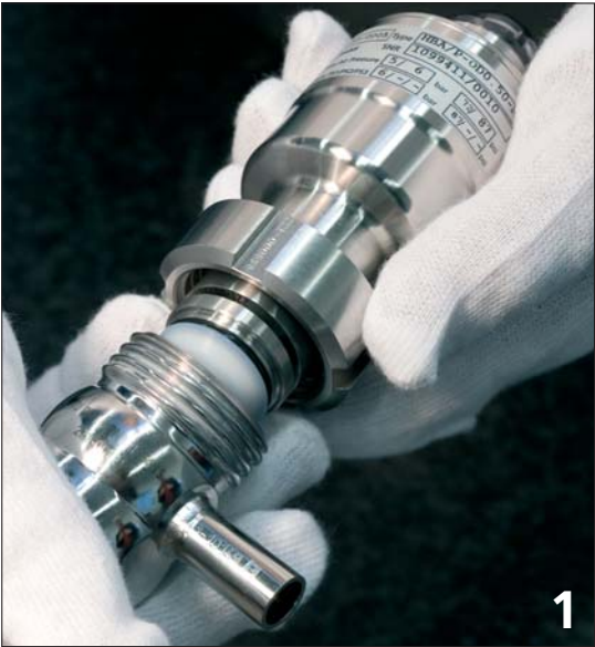
Slacken groove nut and withdraw valve insert
