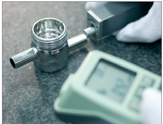
Quality check – Surface measurement determining its R a value
