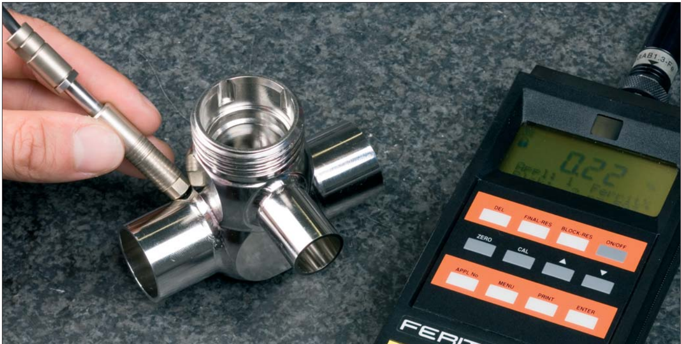
Ferrite content measurement is part of the quality assurance procedure
