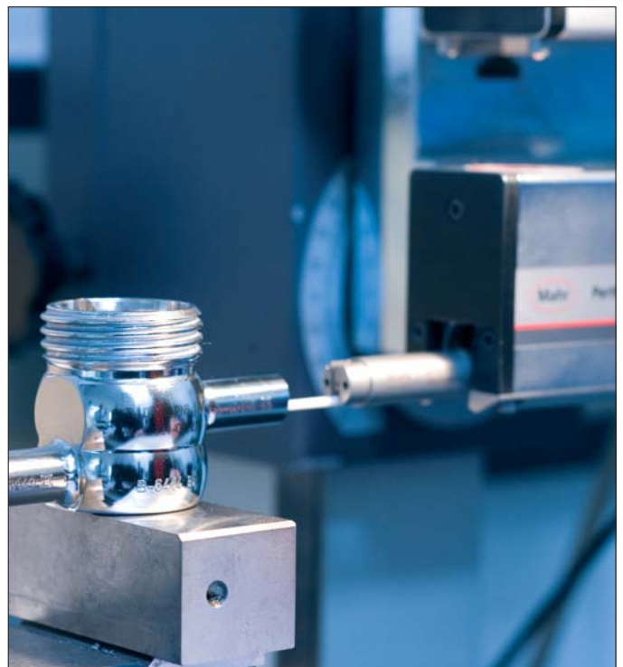
Surface finish: fine-machined, R_a 0.8 \mu m
