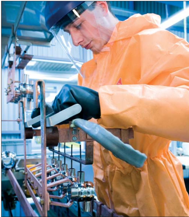
Workpieces on a holder being dipped in an electropolishing bath
