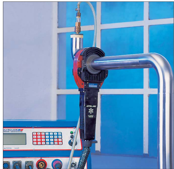
WIG orbital welding system with enclosed cartridge system
