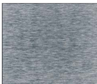
Surface finish: fine-machined and grinded, R_a 0.2 \mu m
