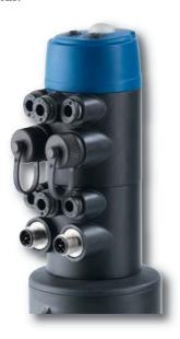
The T.VIS® P-1 / P-20 is a compact position controller for pneumatic valves. By specifying a setpoint (4-20 mA), transferred e.g. by the PLC, the process valve can be brought to any position. The position is detected by a position sensor with a resolution of 0.01 mm and adjusted by 2 integrated solenoid valves.
